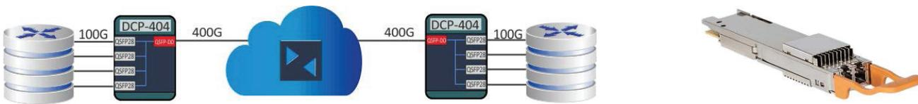
OpenZR+ is currently only defined for amplified line systems. OIF 400ZR is defined for both amplified as well as un-amplified configurations. The Application Mode 2 (OIF app code 0x02) corresponds to the un-amplified OIF 400ZR configuration.
